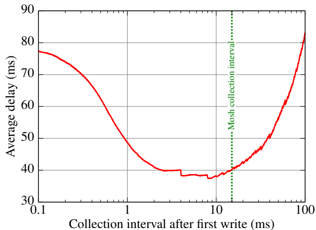
Figure 8: Average protocol-induced delay from varying collection interval (with frame interval of 250 ms)
